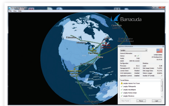
Barracuda Earth - the graphical real-time 3D network monitoring utility of the Barracuda NextGen Control Center, provides a status overview of all VPN site-to-site tunnels.
